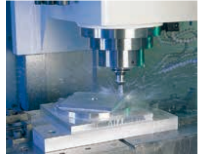
CTS (Coolants Thru. Spindle)
