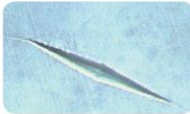
Spherical Cast Tungsten Carbide 160 \mu m: picture with Knoop indentation under 1 kg (2.2lb.load.)
