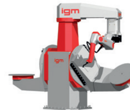
Compact system RSX with rotary arm RST and L-manipulator RWM2 designed for welding systems with one or two stations, load capacity from 500 to 1,000 kg per station
