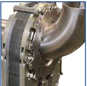
Adjustable protection disc for gas protection
