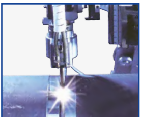
Torch module "V2 Narrow Gap", for wall thicknesses up to 75 mm
