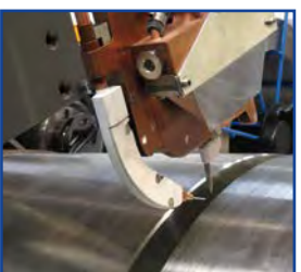
"Narrow groove" torch module for wall thicknesses up to 300 mm
