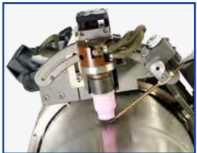
Torch block with AVC/OSC cross slides and adjustable wire guide
