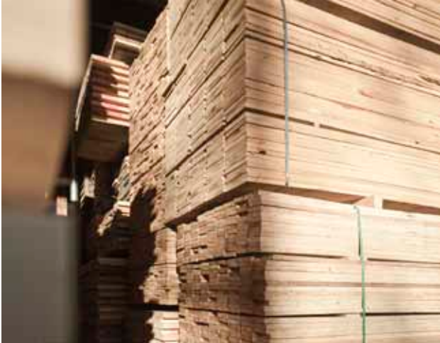
PEFC or FSC® C119602 - certified lamellae undergo machine strength grading and are sorted according to surface quality
