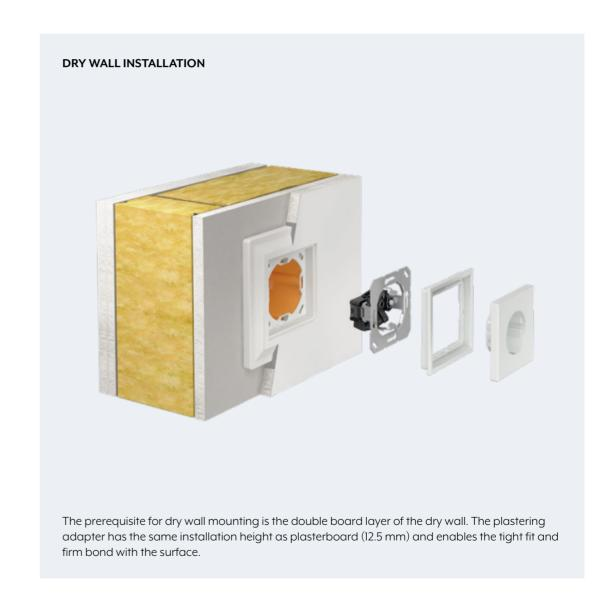
The "Brickwork / Dry Wall" video explains the individual installation steps. jung.de/lszero
