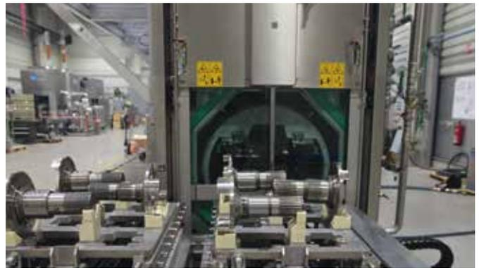
**Automated cleaning of planetary carriers in a line production with robotic loading**
