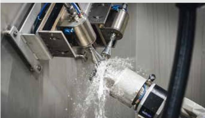
**Robot-assisted component guiding to a permanently mounted nozzle system**
