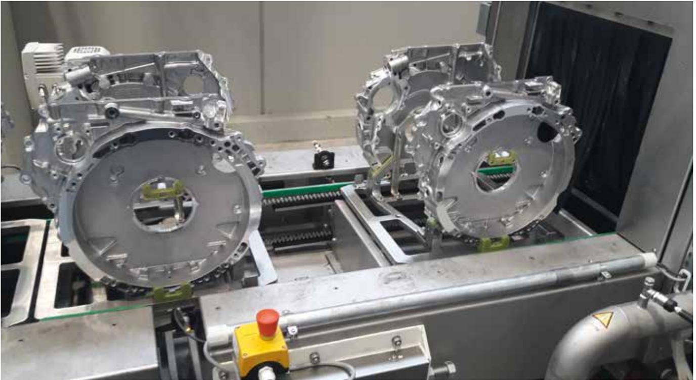
**Efficient cleaning of cast aluminium components with complex geometries**
