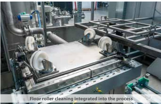
Floor roller cleaning integrated into the process
