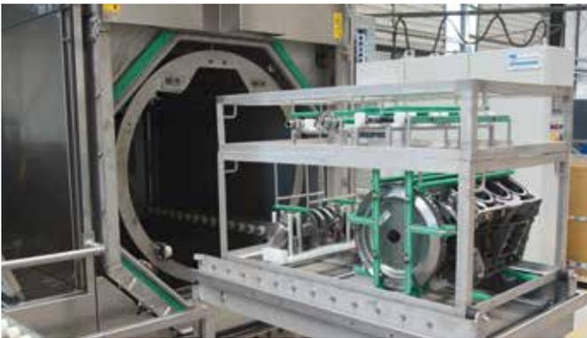
**Cleaning of different engine components in one system**
