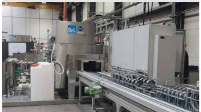
**Cleaning of high-quality gearbox components without residue in customised baskets**
