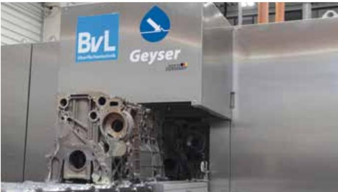
**Deburring and cleaning of an entire engine block**
