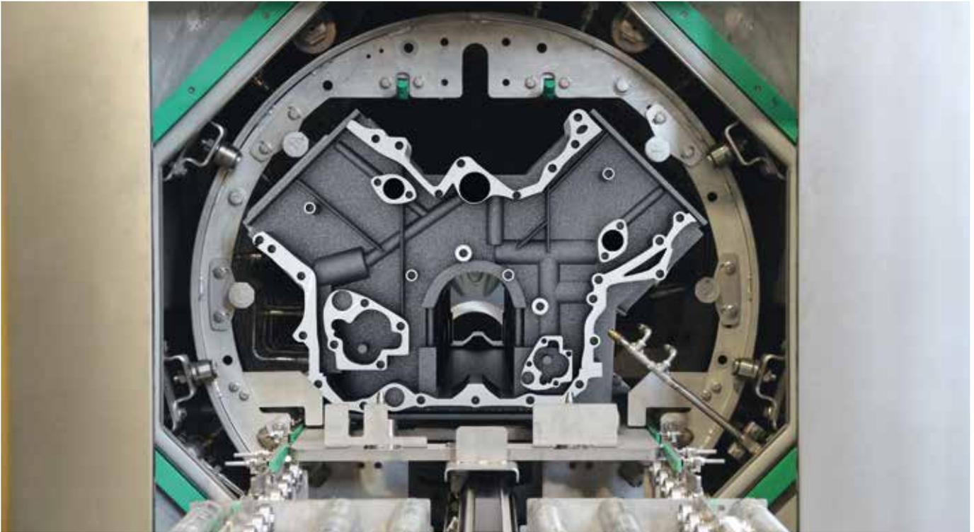
**Targeted external and internal cleaning of cylinder blocks and cylinder heads**
