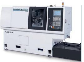
**THE MANURHIN K'MX 532 TREND** is designed for productive machining of parts for bars with a maximum diameter of 32 mm. With a spindle bore diameter of 37 mm, no modification of the end of the bar for bar feeder collet is needed. The machine comes standard with two electrospindles, each with a maximum speed of 10,000 rpm and with a rotary guide bush, synchronized by pulleys and belts from the main spindle. Five linear axes (X1, Y1, Y2, Z1, Z2) two rotary axes (C1, C2).
