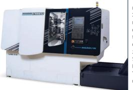
**THE MANURHIN K'MX 632** is designed for productive machining of parts for bars with a maximum diameter of 32 mm. With a spindle bore diameter of 37 mm, no modification of the end of the bar for bar feeder collet is needed. The machine comes standard with two electrospindles, each with a maximum speed of 10,000 rpm and with a rotary guide bush, synchronized by pulleys and belts from the main spindle. Six linear axes (X1, X2, Y1, Y2, Z1, Z2), two rotary axes (C1, C2).
