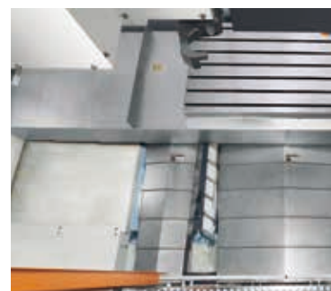
Bottom guarding flush + Screw chip removers
