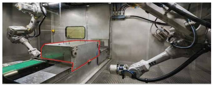
Workpiece holder cleaning as optional component
