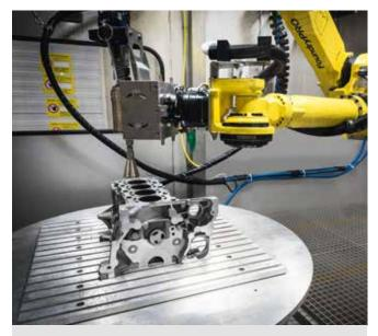
**Robot-assisted high-pressure water tool** for large effective dimensions
