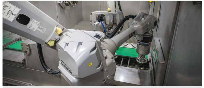
The deburred component is placed on the cleaned workpiece holder.This prevents the component from becoming contaminated again by residues on the workpiece holder.
