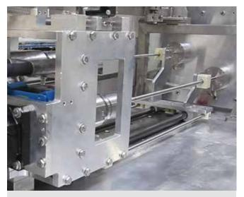
High-pressure lances Targeted deburring of oil and water channel holes
