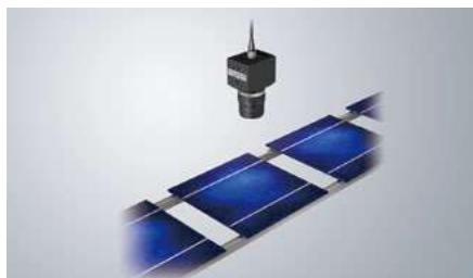
Inspection of broken solar cell patterns
