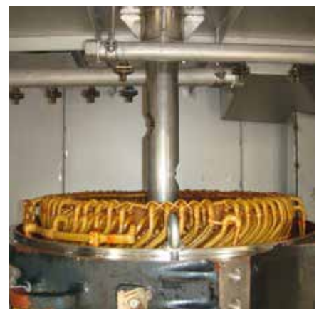
Lance system for internal cleaning of the stators
