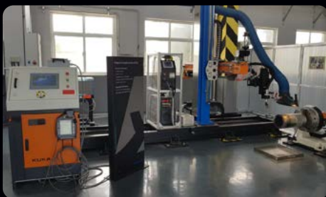
PTA & Laser Cladding work cell
