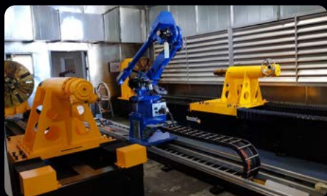
Designed & Built robotic thermal spray cell
